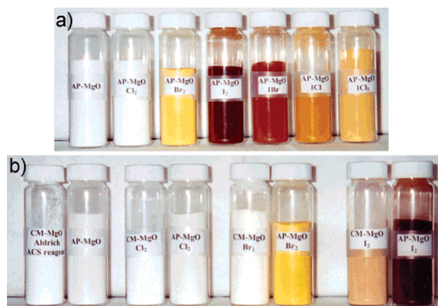
Figure 1. Photographs of (a) nanoscale AP-MgO/X 2 and (b) AP-MgO/X 2 and their bulk counterparts (CM-MgO/X 2 ) synthesized at identical experimental conditions.
